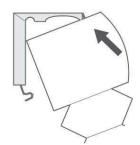
Situate the front lip of the headrail into the front hook of the bracket.
