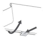
To remove the blind from the brackets, insert a flat head screwdriver into the tab protruding from the bottom of the rail, then gently pry it back while tilting the back of the rail downwards. Repeat this carefully for each bracket to release the rail.
