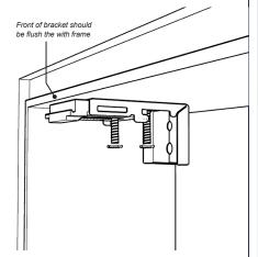
**Outside Mount:** Outside edge of the brackets should be positioned at least 1/2" to the outside of the headrails end mark. Use wall anchors for a secure hold. Mark the position of the bracket as illustrated.
