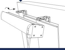
push shade into spring brackets till springs compress
