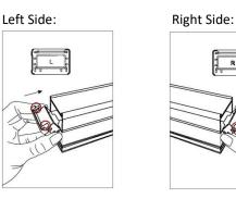
To install Bottom Rail Left and Right End Caps, match the flat side of end caps with the bottom rail of your shade (For bottom rail end caps, left / right side are the same). By using the flat surface on end caps, push fabric/ stiffener against end of rail and slide end caps into side of rail.
