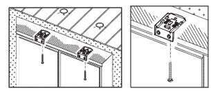
Make sure both brackets are aligned. "L" shape opening should be facing down, with longer side against top of the window opening.
