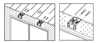
Make sure brackets are aligned. "L" shape opening should be facing down, with shorter side against the wall.
