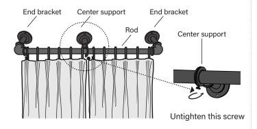
Firmly hold end bracket with one hand and slowly pull the rod out of the end bracket with the other hand. Gently nudge if necessary. Do not twist the rod to avoid misalignment. Rod adapter will stay on the end bracket.
