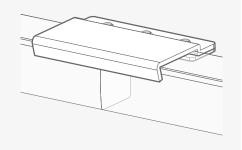
If your Curtains are over 2,500mm wide then you will be supplied with 2 headrails, which are joined together in the middle using the joining plate supplied.
