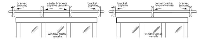
2. Mark screw locations using a pencil. It is recommended that the screws be driven directly into a wall stud. However, if this is not possible or practical, drywall anchors have been provided. Drill starter holes for the screws or screws & anchors.
