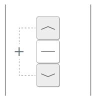
Hold the OPEN and CLOSE buttons on the remote at the same time until the motor 'jogs' briefly.
