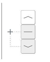
Hold the CLOSE and STOP buttons until the motor 'jogs'. The motor is now deleted from all channels.
