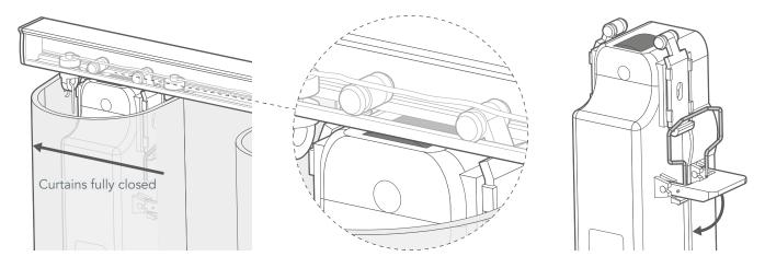
Take the runner you detached and hook it into place in the rail just as before, then clip it back into its mount on the side of the motor. Push the motor and curtain along the rail so that the curtains are in their fully closed position before locking the retaining clips on the sides of the motor.
