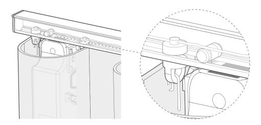
Lift the motor up behind the curtains and hook the runner that's still attached into the channel on the underside of the curtain rail.
