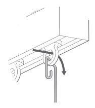
Insert the hooks into the plastic eyelets in the headrail.
