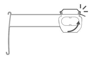
Rest the foremost of the lips on the headrail in the front lip of the bracket.
