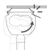
Then twist the back of the headrail upwards until it snaps into place in the rear hook of the bracket.
