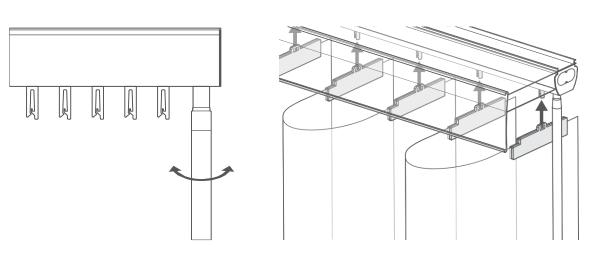
Twist the control wand to turn the hooks so that their 'open' part is facing into the room.
