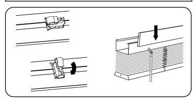
Evenly space valance clips on backside of the valance. For Inside Mount, attach valance before blind installation. For Outside Mount, attach valance after blind installation.
