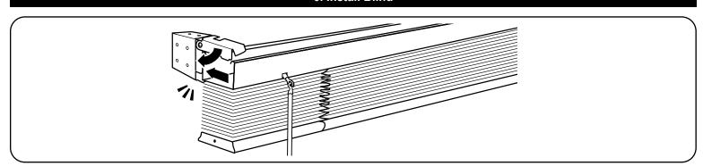
Slide blind into bracket and snap door closed. Use both hands on the bottom rail to lift or lower blind. Rotate wand to tilt slats. Blind slats should be tilted open prior to lifting and lowering.
