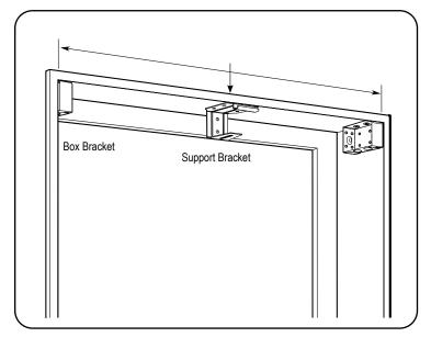
Place box brackets into corners of the window frame. Evenly space support brackets between box brackets, away from ladder cords. Mark bracket positions.
