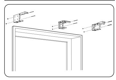
Drill pilot holes and install brackets using screws provided. Wall anchors may be required for secure attachment (not included).
