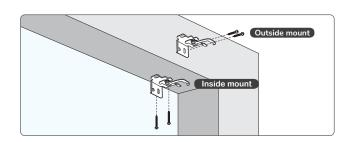
Mark the location of the screws using brackets as a guide. Drill holes for the screws and install the brackets (depending on the material of your walls, you might need to use drywall anchors).
