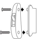
Tension Device & Bracket for Outside Mount
