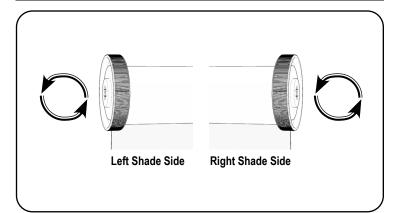
To **lower tension or speed**, turn the left side wheel towards the back of the shade. To **add tension or speed**, turn the left side wheel towards the front of the shade while holding the bottomrail.
