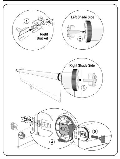
DO NOT REMOVE THE RED PLASTIC CLIP. IT WILL DISENGAGE ONCE THE BRACKET HAS BEEN INSTALLED.
