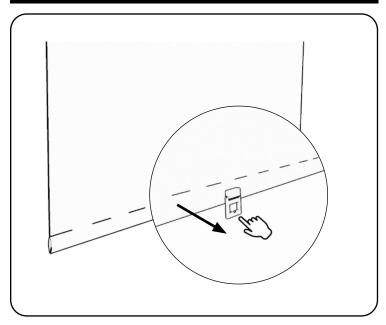
Pull the bottom handle and let go to lock it into the desired length.
