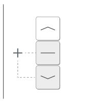
Hold the CLOSE and STOP buttons until the motor 'jogs'. The motor is now deleted from all channels.
