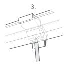
Hold the rail up to the fitting surface and mark out the screw holes with a pencil.
