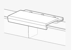
If your Curtains are over 2,500mm wide then you will be supplied with 2 headrails, which are joined together in the middle using the joining plate supplied.
