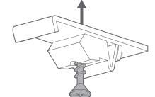
Clip the brackets onto the rail, spaced out as described at the start of this guide..
