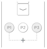
Press and hold the P1 and P3 buttons together until the motor 'jogs'. The motor is now in configuration mode.
