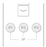
Press and hold either P1, P2 or P3 until the motor 'jogs'. The new intermediate stop-point is now set to that button.
