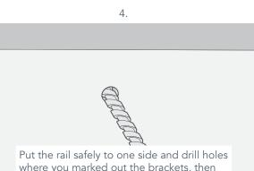
where you marked out the brackets, then insert a hollow wall anchor into each hole.
