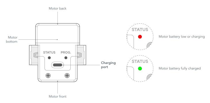
The motor has a USB-C charging port on the bottom. To charge the motor's battery, simply plug the charging cable into the charging port. A full charge typically takes around 8 hours if the battery is fully depleted. Whilst charging, the STATUS light on the bottom of the motor will glow red, then change to green when fully charged.
