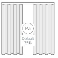
By default, pressing P1 will move the curtains to 25% closed, P2 to 50% closed and P3 to 75% closed, but these positions can be changed if preferred.
