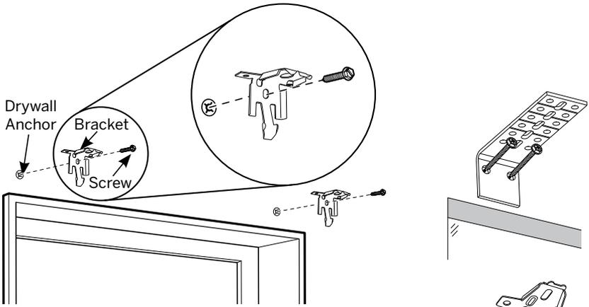
STEP 2: INSTALLING THE BRACKETS
