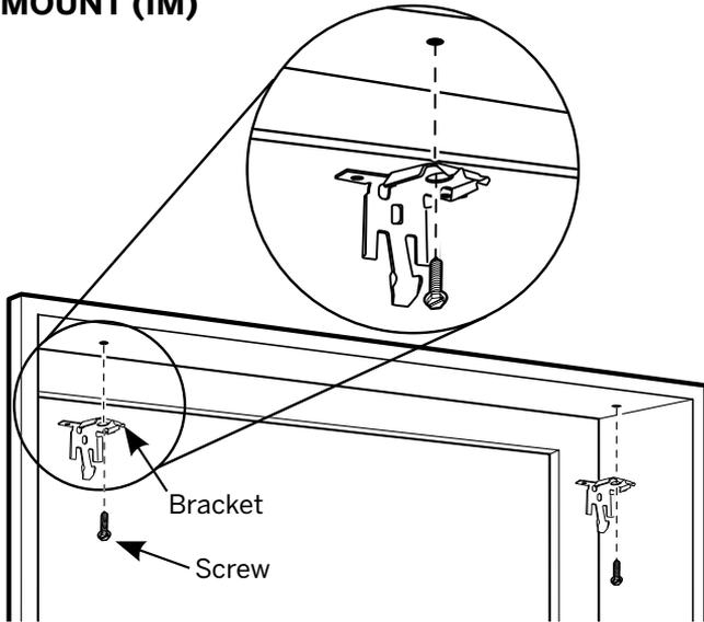
**STEP 2: INSTALLING THE BRACKETS**
