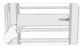
Separate the louver from the nylon pin and remove the louver from the panel.
