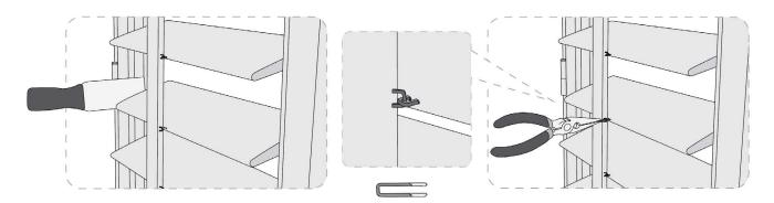
Using a putty knife or your finger depress the spring-loaded pin. Slide the louver down, aligning the hole in the louver's center with the spring-loaded pin until it locks into place.
