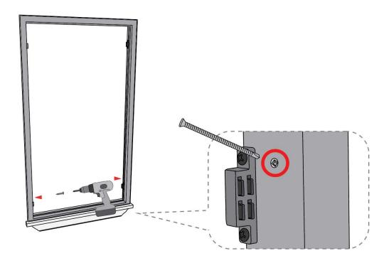
If your windows have more than one panel, close the shutter panels, they should be even across the top in the frame. If the panels are uneven, shift the frame at the top left or right as needed until the panels are evenly spaced in the frame on all sides.
