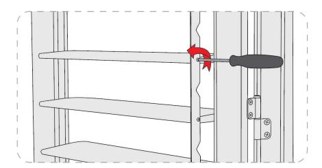
Open the shutter door completely. Using a Phillips head screwdriver, remove the tiny screw and washer attached to the ClearLine strip and remove the broken/damaged louver.
