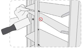
Insert a nylon pin into the louver on the opposite side of where the springloaded pin will enter. Insert the nylon pin side of the louver into the stile making sure the staple holes are facing toward the tilt-rod.
