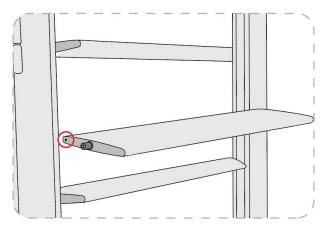
Insert a nylon pin into the louver on the opposite side of where the spring-loaded pin will enter. Insert the ClearLine side of the louver into the stile, making sure the ClearLine hole faces the ClearLine strip.
