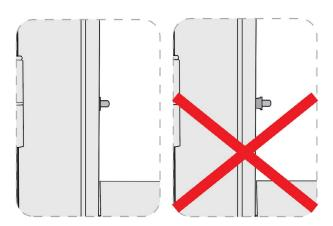
Remove the nylon pin from one side and replace with a spring-loaded pin included in the hardware kit. Make sure the pin base is flush with the stile.
