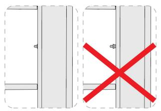
Remove the nylon pin from one side and replace with a spring-loaded pin included in the hardware kit. Make sure the pin base is flush with the stile.
