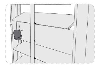
If the broken/damaged louver is not at a tension screw location, use a box knife to make a 1-inch horizontal cut in the center of the louver closest to the stile.
