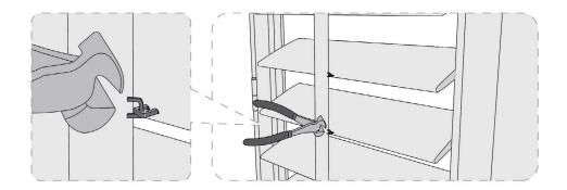
Using wire snips or pliers, cut or pull out the staple in the broken/damaged louver.
