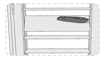
If the broken/damaged louver is not at a tension screw location, use a box knife to make a 1-inch horizontal cut in the center of the louver closest to the stile.
