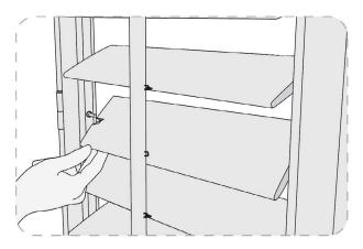
Separate the louver from the nylon pin and remove the louver from the panel.
