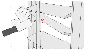
Insert a nylon pin into the louver on the opposite side of where the springloaded pin will enter. Insert the nylon pin side of the louver into the stile making sure the staple holes are facing toward the tilt-rod.
