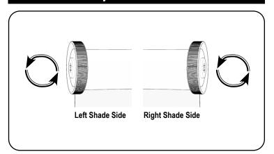
To lower tension or speed, turn the left side wheel towards the back of the shade. To add tension or speed, turn the left side wheel towards the front of the shade while holding the bottomrail.
