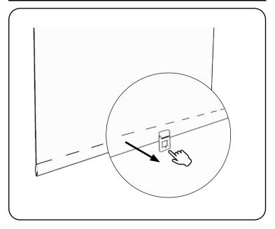
Pull the bottom handle and let go to lock it into the desired length.
