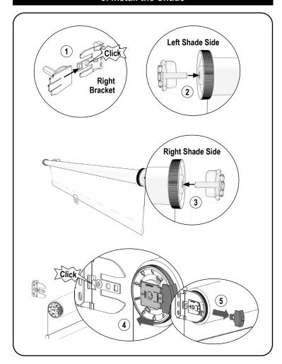
DO NOT REMOVE THE RED PLASTIC CLIP. IT WILL DISENGAGE ONCE THE BRACKET HAS BEEN INSTALLED.
