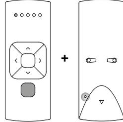
**23.3** All blinds in the selected channel will start stepping, indicating program mode has been activated. All blinds can be copied to a new channel on the same remote or a different remote. Select a new channel on the (new) remote.
