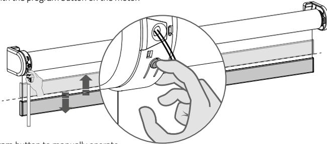
**20.1** Hold the **program** button to manually operate the blind. The blind will move as long as the button is being pressed. (max. 15 sec.)
