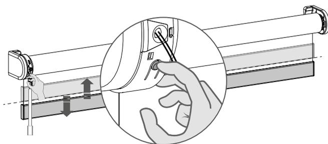
**18.1** Press the program button on the motor to activate program mode.
