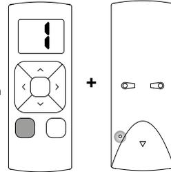
**24.3** All blinds in the selected channel will start stepping, indicating program mode has been activated. All blinds can be copied to a new channel on the same remote or to different remotes. Select a channel on a (new) remote.
