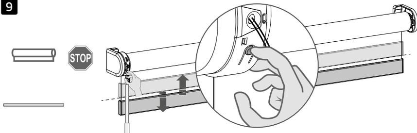
**i** Save the position by pushing the button until the blind moves up and down.
