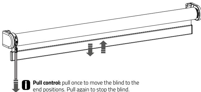
**i Pull control:** pull once to move the blind to the end positions. Pull again to stop the blind.
