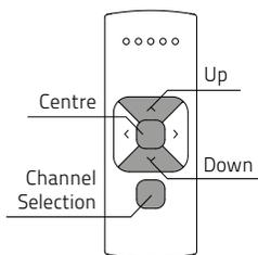
**i Remote control:** Choose the channel with which the blind has been paired using the **channel** button. Press the **up** or **down** button to operate the blind. Press the **centre** button to stop the blind.
