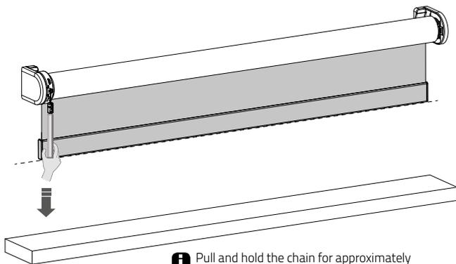
**i** Pull and hold the chain for approximately 7 seconds until the blind moves up and down.
