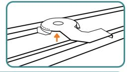
While holding the track in place, swing each bracket 90 degrees to the left and lock the track onto the bracket.
