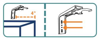
After mounting the brackets, slide the track onto the brackets with the lever facing outward toward the window opening.
