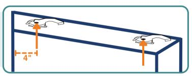
After mounting the brackets, slide the track onto the brackets with the lever facing outward toward the window opening.
