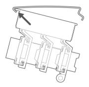
Rest the front lip of the headrail in the front lip of the bracket.
