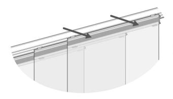
Simply press the Velcro strip on the back of each panel onto the corresponding strip of each glider.
