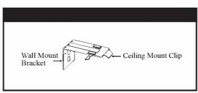
A. OUTSIDE MOUNT: Mount on a vertical surface (wall, window, or door frame) STEP 3A. The length of your blind is the exact distance from the top of your
