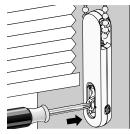
**CAUTION:** Do not overtighten the mounting screw. This can prevent the UCT from functioning properly and increase bead chain wear.
